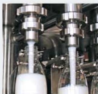
New generation of hygienic filling valves with precise dosing
