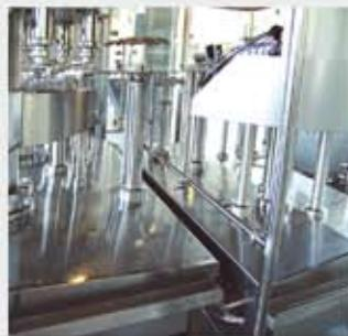
Inclined support plates to lead-off washing liquids quickly and completely
