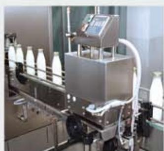
Weight and cap monitoring system with an automatic rejection device
